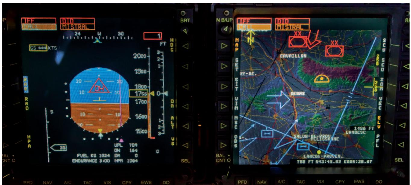
Pilot cockpit with PFD and tactical display in elevation mode
