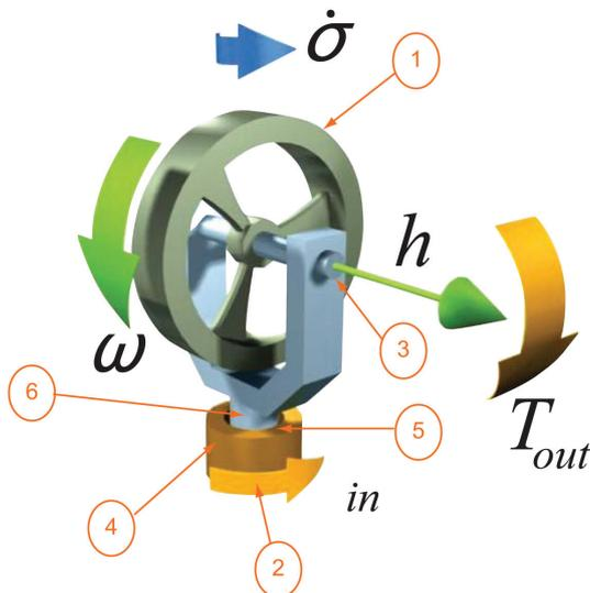
The kinetic momentum is fulfilled by the wheel (1) at constant speed. The precession of the wheel is fulfilled by the gimbal motor (2). The output loads are supported by the ball bearing of the wheel (3) and of the gimbal (4). An angular encoder allows the measurement of the gimbal position (5). The signals and power are led to the wheel through sliprings (6).
