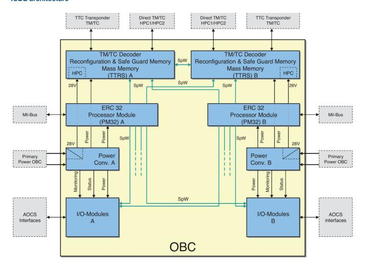
A Cross Coupling Network implementing IEEE1355/ SpaceWire links and a cross strapping network implementing general interface allow ICDE-NG internal communication between the main and redundant modules but such that the ICDE-NG control is hardware exclusive between two processor modules.
