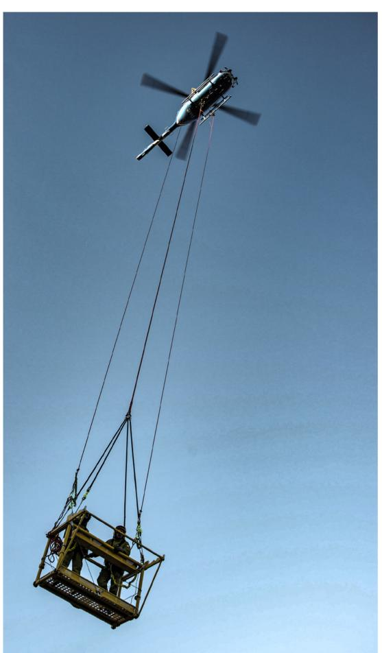
Light basket, both dropped and suspended, can be used on live wires.
