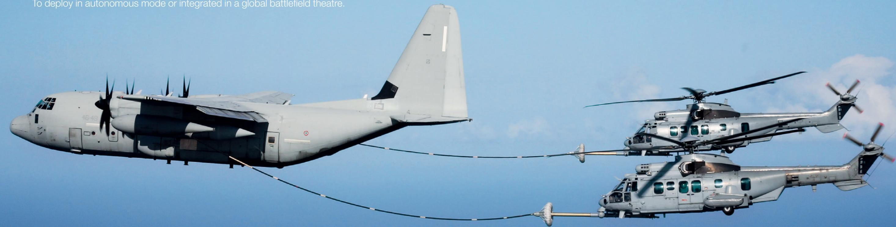
Unrivalled range with up to 3 tons of fuel tank capacity complemented by Air to Air Refueling (AAR), or Hover In Flight Refueling (HIFR) capabilities.
