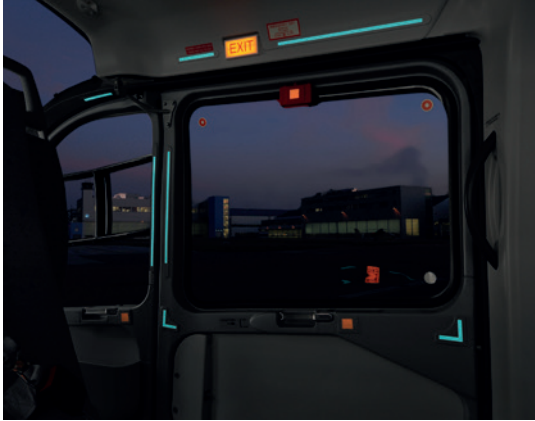
H.E.E.L.S. Helicopter Emergency Egress Lighting System
