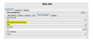
If set to yes, the direct and indirect absorbed solar fluxes are exported only to the h5 file, not to the nwk file. The option "direct/indirect fluxes" is available only if the option "direct flux only" is set to no.
