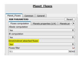
If set to yes, the direct and indirect absorbed planet fluxes are exported only to the h5 file, not to the nwk file. The direct/indirect albedo and infra-red fluxes are calculated only if the albedo and IR computation are enabled respectively.
