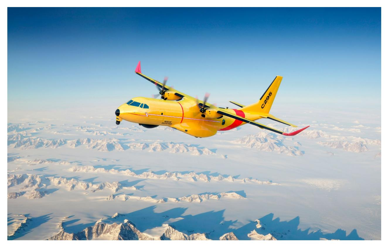
The C295W version is equipped with winglets, giving it the capability to transport more payload over longer distances, with fuel savings of approximately 4% and increased safety margins for hot-and-high conditions, as well as in mountainous regions.
