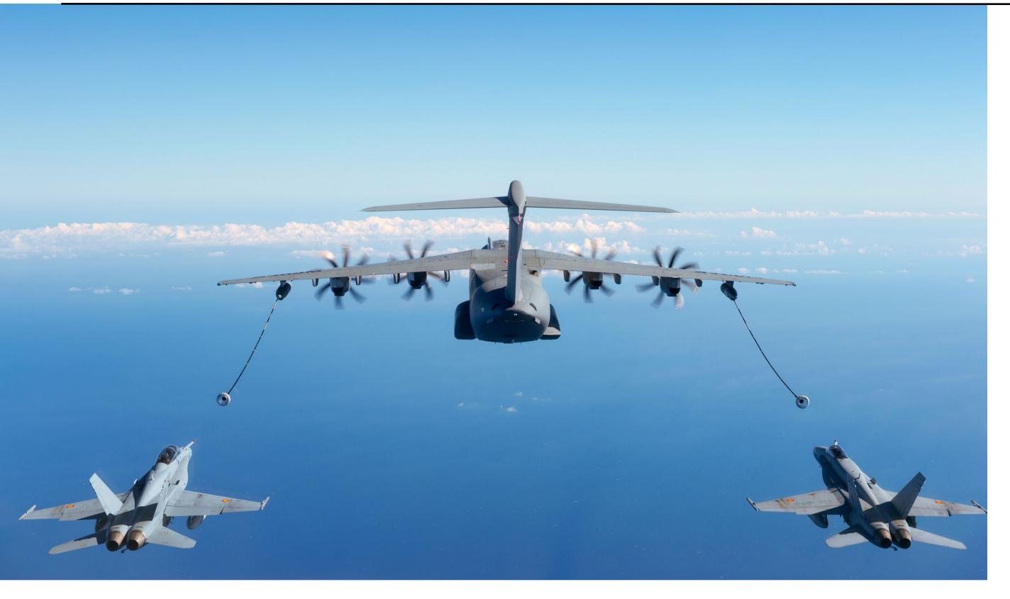
Multiple challenges were encountered during the A400M's development. Among them were gearbox issues with the Europrop TP400 engines – the largest turboprop powerplants developed for operational use in the West – which limited the aircraft's operational capabilities, and were treated first with a temporary fix, followed by a permanent solution. Shortfalls in mission performance also were addressed with retrofits and upgrades.
