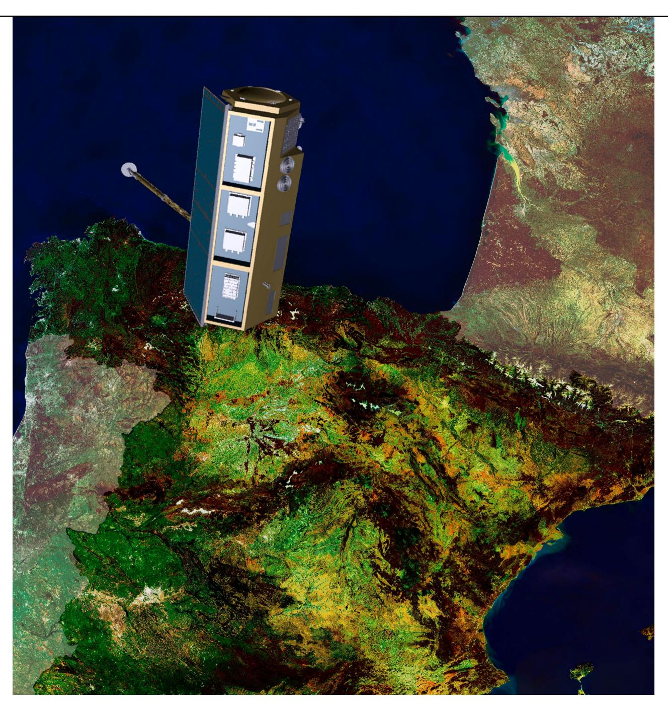
The Airbus-built SARah-1 next-generation reconnaissance satellite for the German Bundeswehr was launched in 2022. As the successor system, it replaced the SAR-Lupe system and offers significantly enhanced capabilities with its active phased array antenna for fast and flexible radar imaging. Airbus led the development of the radar technology, launch, calibration, and operational readiness of the satellite, demonstrating its continued technological leadership in SAR.
