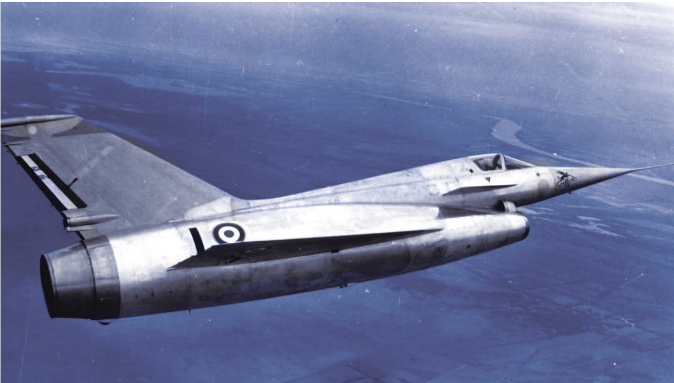
The Nord 1500 Griffon was the world's first supersonic aircraft equipped with a ramjet.
