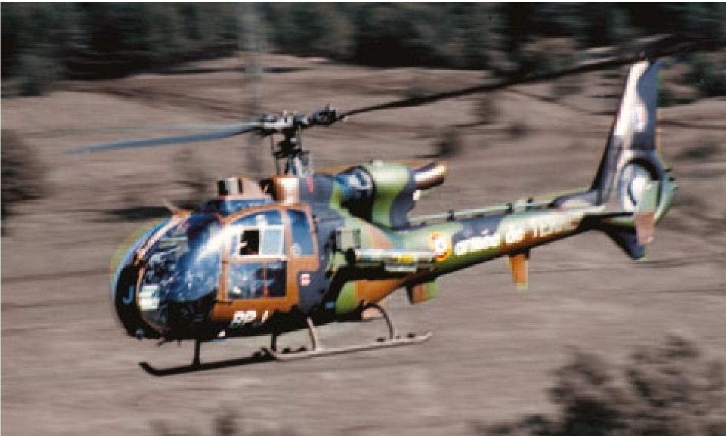
APRIL 12, 1967 - MAIDEN FLIGHT OF THE SA.340 GAZELLE The SA.340 Gazelle light helicopter was – like the Puma and Lynx – the result of cooperation with Westland. It was the first helicopter equipped with an encased tail rotor, known as a fenestron. 1,255 units of this helicopter were built.
