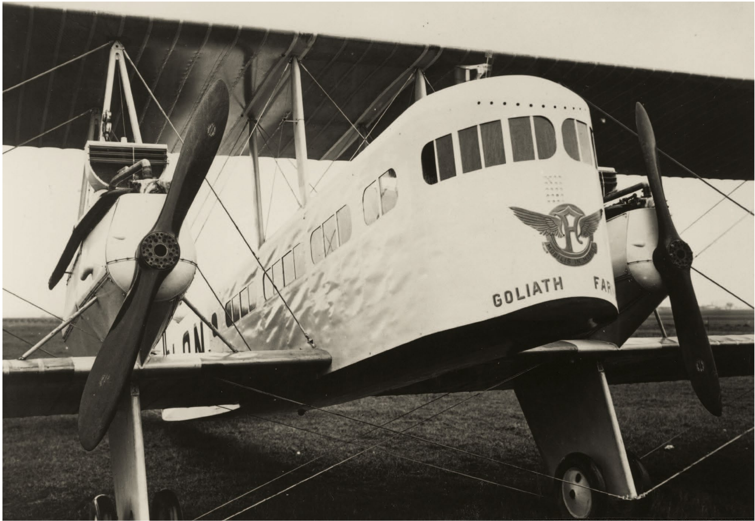
1919 - AIR LINK BETWEEN PARIS AND LONDON The Farman F.60 Goliath set out on the first international route in civil aviation (Paris – London) in 1919. The aircraft, which was originally designed as a heavy bomber, was later used exclusively as a passenger plane.
