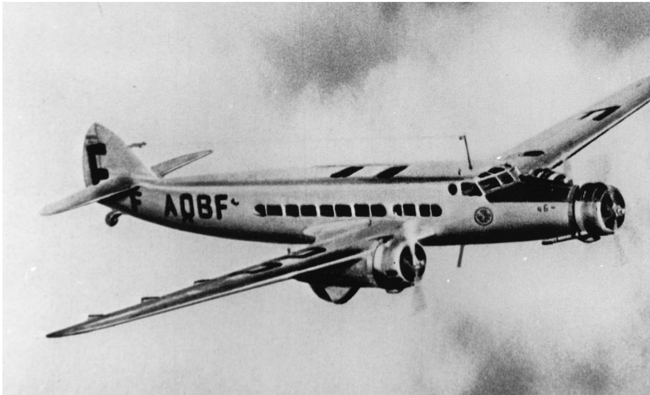
AUGUST 29, 1935 - MAIDEN FLIGHT OF THE DEWOITINE D.338 The Dewoitine D.338 was a triple-engine passenger plane similar to the Ju 52. It was used both in European transport and for long-haul flights to Indochina.
