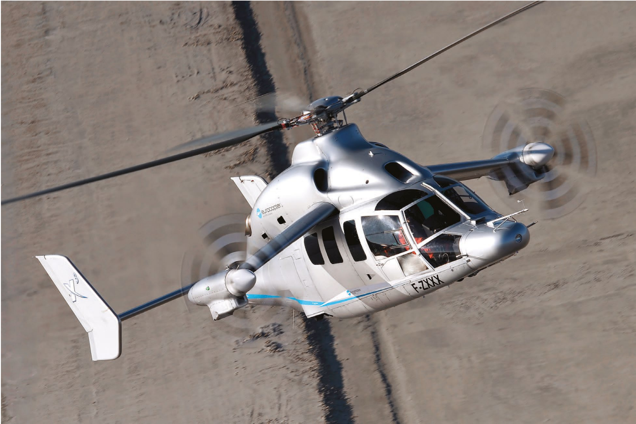
SEPTEMBER 27, 2010 - X3 TEST FLIGHT Eurocopter started test flights of the X3 demonstrator for its innovative High-speed, long-range Hybrid Helicopter (H3) concept, which combines excellent vertical takeoff and landing capabilities with fast cruise speeds of more than 220 kts.
