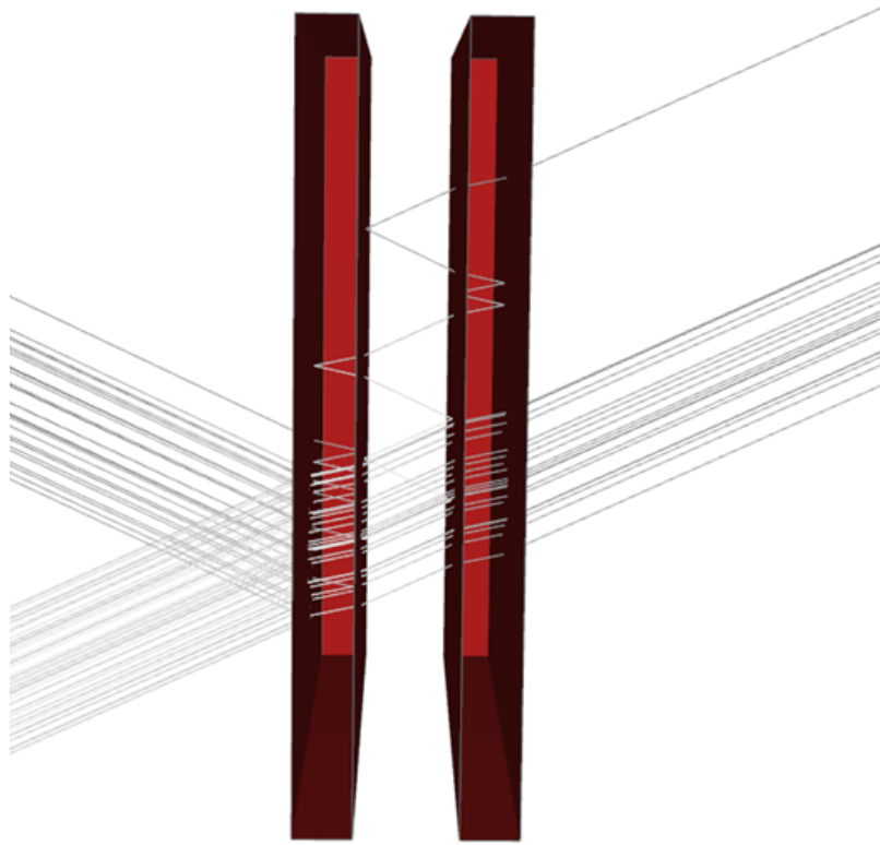
Ray tracing through two glass plates – partial reflection and transmission
