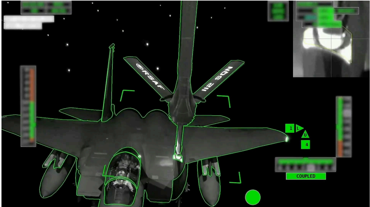
RSAF A330 MRTT refuels a RSAF F15 via A3R during night © Airbus SAS 2022
