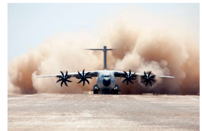
▲ The A400M's unpaved runway capability makes the aircraft a vital asset for supporting special operations and delivering humanitarian aid in the most challenging environments.
