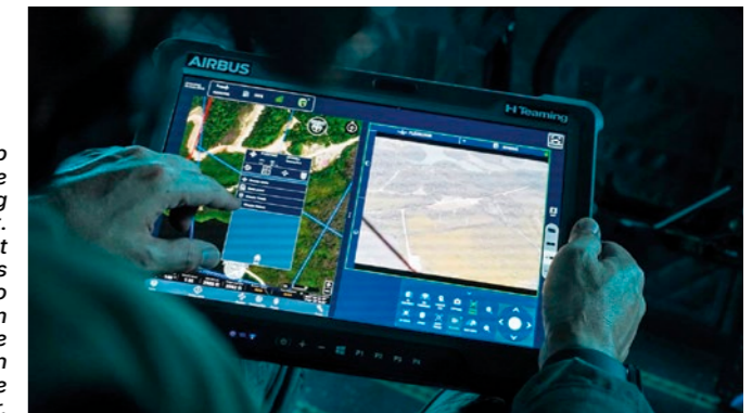
► A close-up view of the HTeaming tablet. The tablet enables the crew to benefit from real-time information from the Flexrotor.
