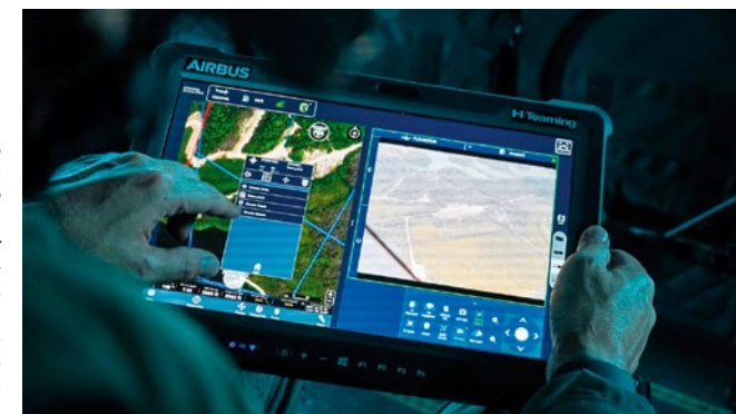
► A close-up view of the HTeaming tablet. The tablet enables the crew to benefit from real-time information from the Flexrotor.
